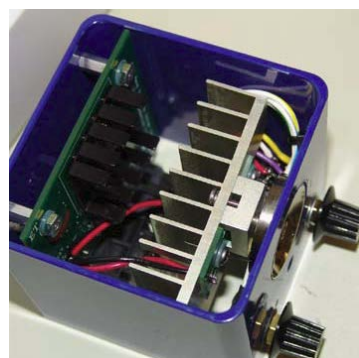
Installed High Power LED Module
